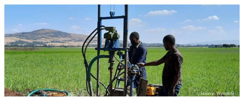
In many areas of the Ethiopia, people have been using traditional techniques of water drilling in the hope of finding groundwater. The problem with manual drilling is that it poses high risk for drillers, and it is not effective with hard rock surfaces.
